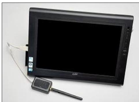
Secure the RF communication module to the tablet or PRO+ computer using the hook-and-loop patch. The tablet is now ready to communicate with the simulator wirelessly. For information about the signal strength indicator, go to the "Working with UNI" section.
