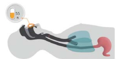
Alarm may alerts when over-pressure is applied on incisors
